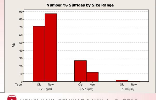
17% more sulfide inclusions in the 1 to 2.5 micron (SMALL) range for steel produced using the new practice.
