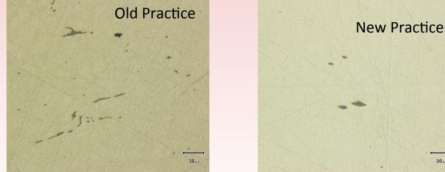
Even at the same sulfur levels (to maintain acceptable machinability), the new steelmaking practice results in small, globular sulfides with a complete lack of large, eutectic sulfides. Eutectic sulfides tend to reduce tensile ductility and toughness.
